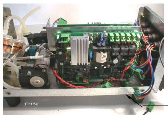
Remove the cover of the analyzer and unplug all the connectors on the elaboration board (see figure).
