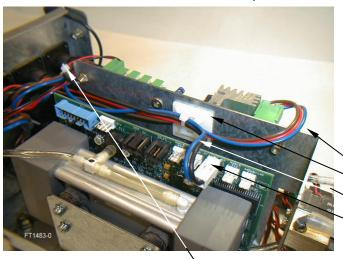
Lock the cables AGS-030 and AGS-080 with a black tie 2.5x100mm.
