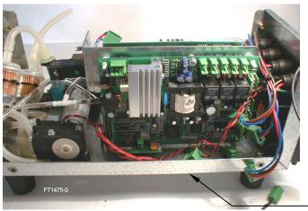
Take the stirrup with the two electronic boards and palce into the frame of the gas analyzer as swowed in fugure.
