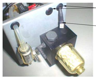
Insert the rubber elements mod. 15419-4 in the holes of the frame as showed.
