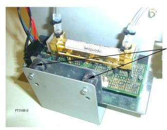
Un-screw the stirrup of the bench from the other stirrup, keeping the two screws TC+ M3x5 ZNT and all the washers M3.
